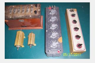
Brief Adjustable capacitors and resistors Description and large single resistors.
