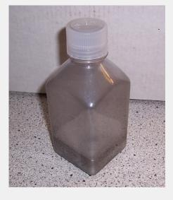
Brief (1) 5 pound bottle of Mercury is available for density demos. Glassware is available in the demo room for use as a vessel for holding mercury on the supply shelf and above the sink
