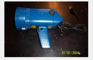
Brief Hand held Strobe light. Digital Description display shows RPM of spinning object in static image. Adjusts in one RPM intervals
