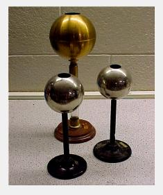
Brief Hollow, conducting balls will pick up Description charge from a Van de Graaff generator. 5A40.? = Induced Charge 5B30.? = Electrostatic Potential
