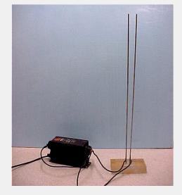
Brief The spark heats the air, which travels upward with accompanying sparks.
