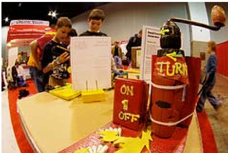
A broken cordless drill becomes a generator. The Little Shop of Physics crew rarely throws anything away; we've always been green.
